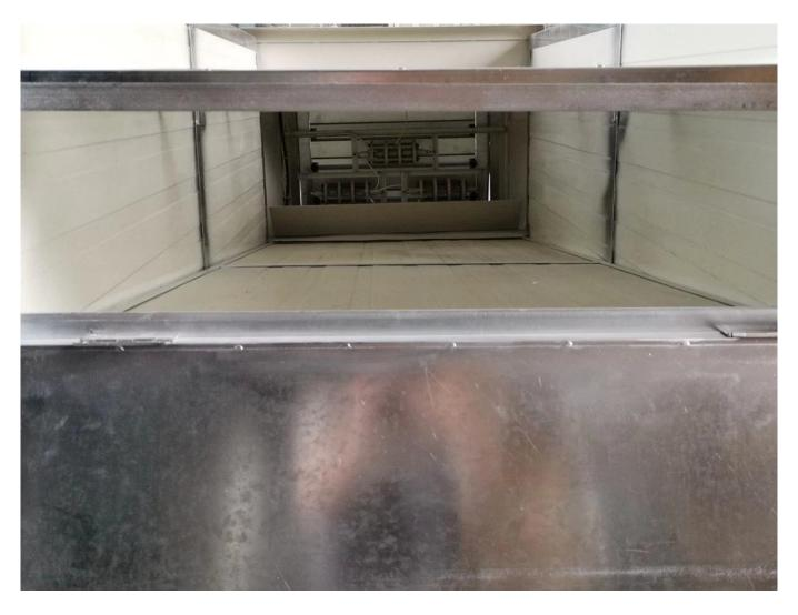
Slope type bottom plate can ensure enough air flow at the tail to ensure the evenness of withering.
