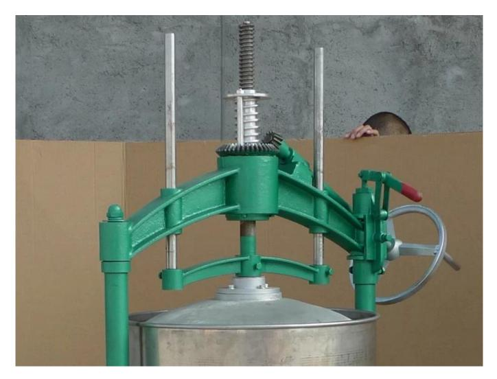
The double arms adopt a double-arm open cover structure, which has a strong bearing capacity and stable operation.
