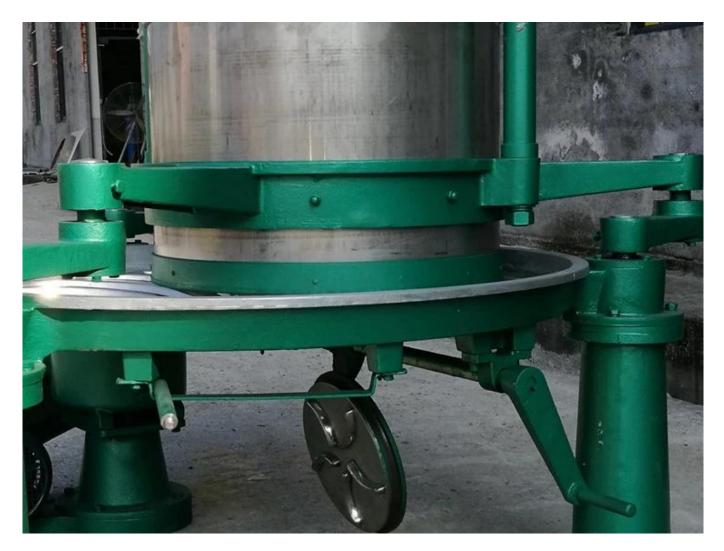
The supporting part of the machine is made of cast iron, which is strong and durable.
