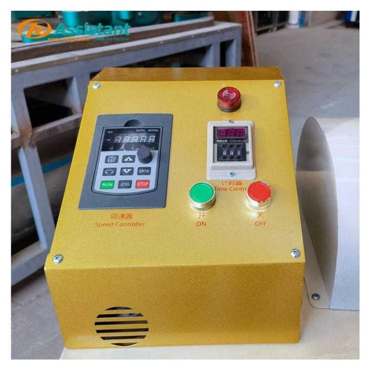
Integrated Chinese and English control panel, with time control function and adjustable speed, is the necessary equipment for the production of high-grade oolong tea.
