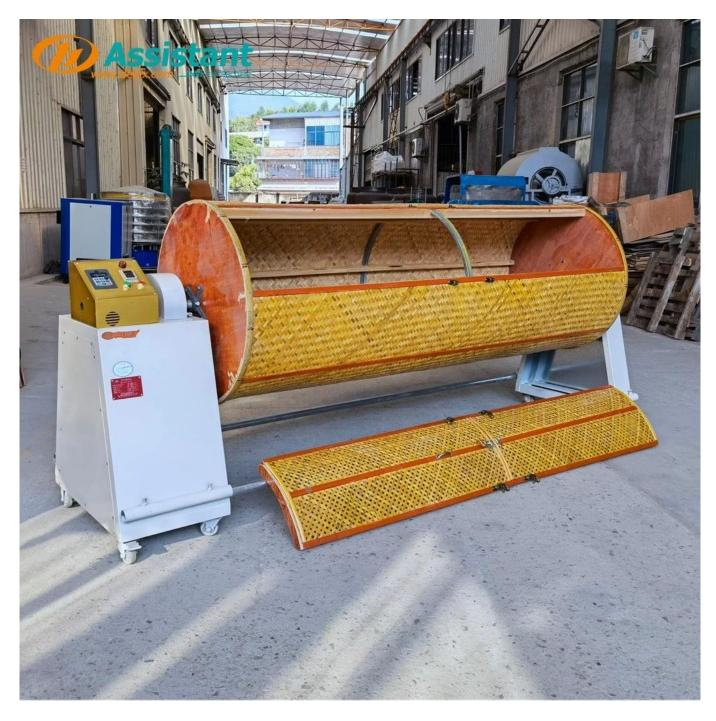
Steel tube and steel ring reinforcement design, the machine runs smoothly, and the body vibration is small.
