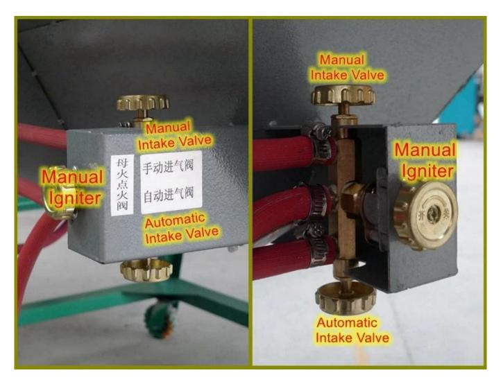
There are three valves at the bottom, which can be manually ignited in case of power failure, so tea leaves are not wasted.
