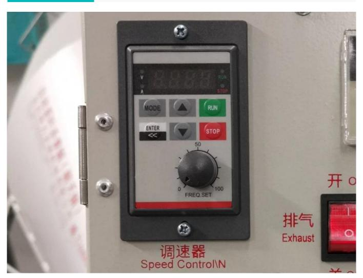
The speed of the tea fixation machine can be adjusted, according to the tea of different producing areas, different speed can be adjusted
