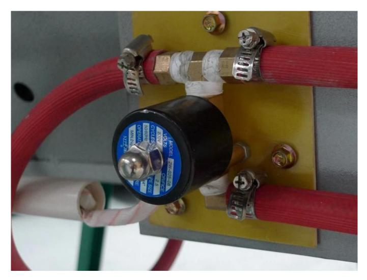
Automatic solenoid valve design, heating automatically starts and stops, the solenoid valve automatically closes when the temperature reaches the set temperature, and the machine stops heating. When the temperature is lower than the set temperature, the solenoid valve opens and the machine reheats, which can save fuel.
