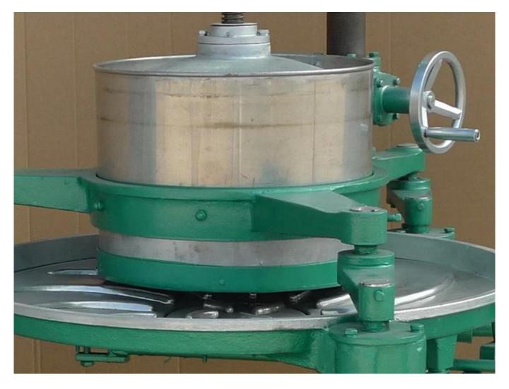
DL-6CRT-35 tea roller table's barrel made of SS304, barrel diameter 35cm, height 26cm, capacity about 8 kg per batch.
