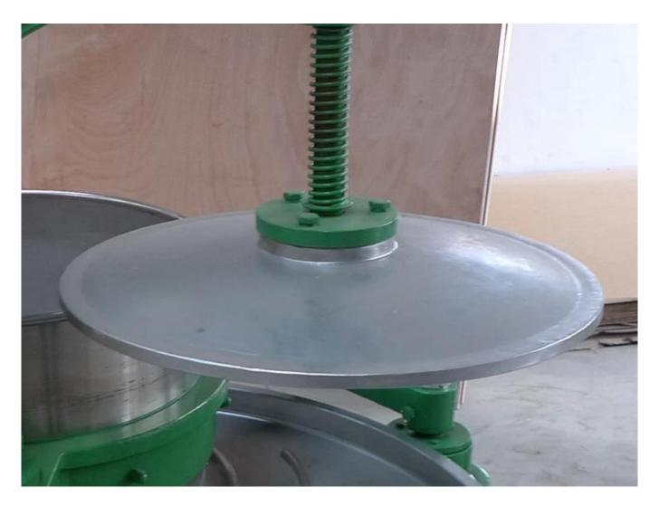
The unique design of the cover of the small and middle rolling machine can be rotated to improve the rate of strip-type tea.
