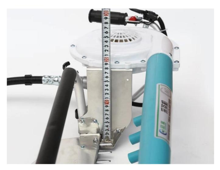
For the tea producing areas with large leaves and the special needs of picking lavender and other flower, we have developed a new type of increased turret, which is 10 cm higher than the conventional one, which greatly improves the picking efficiency.
