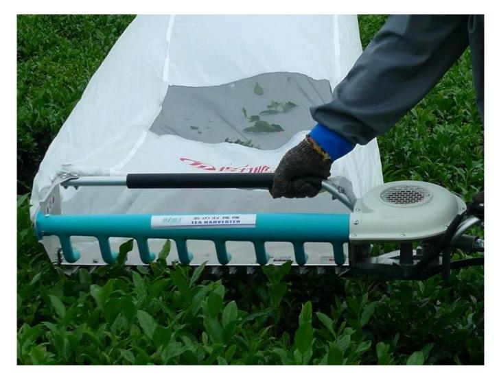
The structure of the blowpipe is optimized. The air volume of each duct is uniform and the wind is more stronger, tea leaf into tea bags faster.
