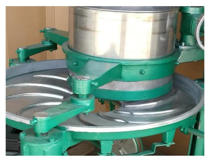
The rolling barrel, rolling disc, and rolling bar are all made of stainless steel, which is hygienic and environmentally friendly.
